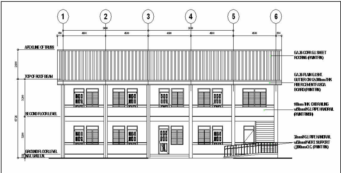
Figure 6: Front Elevation of a 2/3-Storey SBP
